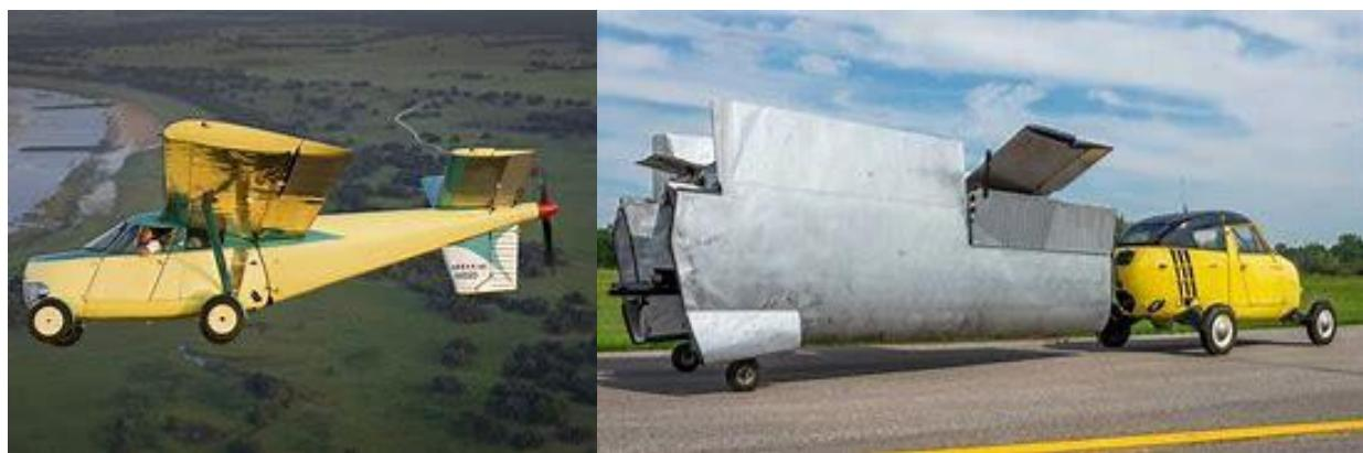
In road use the engine is connected via a three speed manual gearbox to the front wheels—in aircraft mode the rear mounted propeller is driven by a drive shaft from the motor. The high wing and rounded cabin area afforded the pilot-driver excellent visibility, both ahead and down. The wings were easily attached and detached using a hinge type of contrivance. Early advertising said that fitting the wings was “so effortless that a woman could do it without soiling her gloves.”
