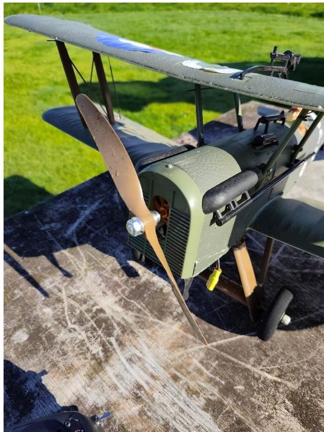
Flight testing of a repowered SE5A. I wasn't happy with the repowered flight time. The performance seemed lack lustre. Might have put the wrong engine in. Couple of flights later and I am seriously thinking that I somehow messed up the power system maths. Nope. Spot what's wrong in this picture. Grant's gonna give me the *propeller* award for that one.
