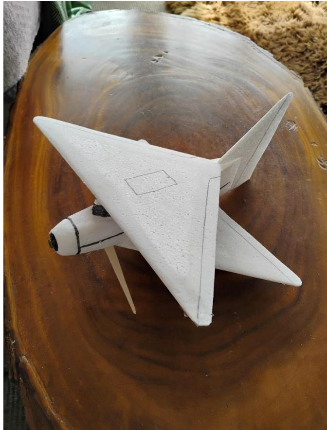
and then they were hot glued onto the remains of my Piper Chub fuselage, suitably shortened. (I've got to be honest, that fat Cub was a squirrelly flier - not enjoyable at all). Then a new tail fin and rudder were made from Depron, and added to the emerging strange shaped beast. Rudder control was pull-pull, and the Depron elevator and ailerons had conventional pushrods.
