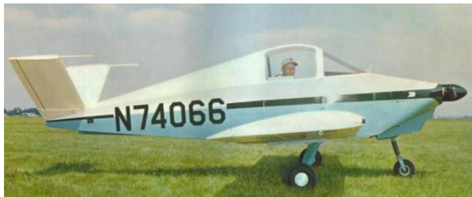
Few tools were needed, a folder and riveter being the major items. Various innovative ideas were incorporated; for instance, the seat adjustment was set so it lowered as it was moved back, allowing for larger pilots. The rails are a structural part of the airframe, instead of being fastened to it, thus saving weight. This design philosophy is carried throughout the aircraft, providing strength without subsequent weight increase.
