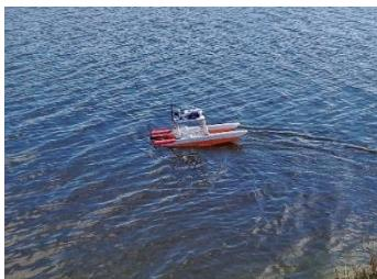
My 3D printed air boat had its first outing. After moving the "C of G" back it went OK. That was, until the motor mount decided to break, flying forward into the hull! So that needs some reinforcing! Beware of stuff on the internet that looks good but has probably never ever been tested!!
