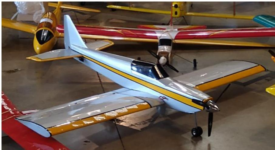
When I got her, she had a 3-blade 14-9 propeller, which I subsequently downsized to a 3-blade 13x8 propeller to drop the current draw and achieve longer flight times. I measured the Watts for both props at various throttle settings and made the change.
