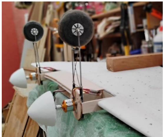
The Mosquito dollys are made from steel reclaimed from a paint roller, also flat steel salvaged from some I found on the road knocked off a street sweeping machine, and plain wire all soldered together solidly. They sit loosely in twin tubes of carbon fibre repurposed from an old fishing rod, and the wheels are slices of hollow pool noodle smeared
