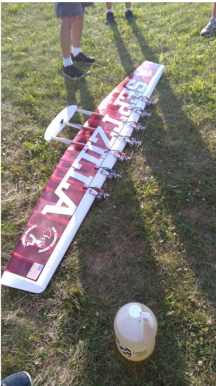
Septzilla the 7 engine Combat model – Fly's well with lots of line tension with all seven engines running
