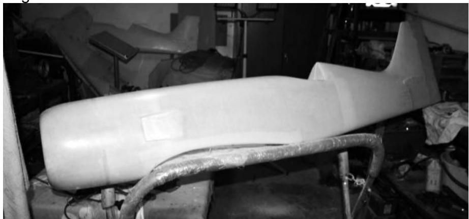
If I was to make another copy I would vacuum bag it as the cloth is not as forgiving as chop strand when laying it up, this eliminating a number of air pockets that needed repair.
