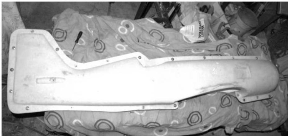
As I had not used glass cloth & epoxy before (all my race car experience was with polyester and chop strand). I did a few experimental lay-ups to get an idea between strength and weight with differing weight clothes/ reinforcement deciding on 200gsm a layer of innegra (56gsm) and another 200gsm
