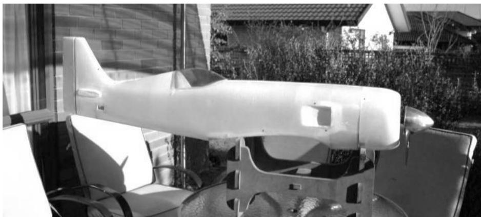
The elevator servos are mounted at the rear to help balance the heavier engine and the exhaust vents are functional and open to help with engine cooling. At this point the fuse is painted, sign written and waiting for wings which are well underway, next newsletter maybe some info on them and a finished plane for the November club night.
