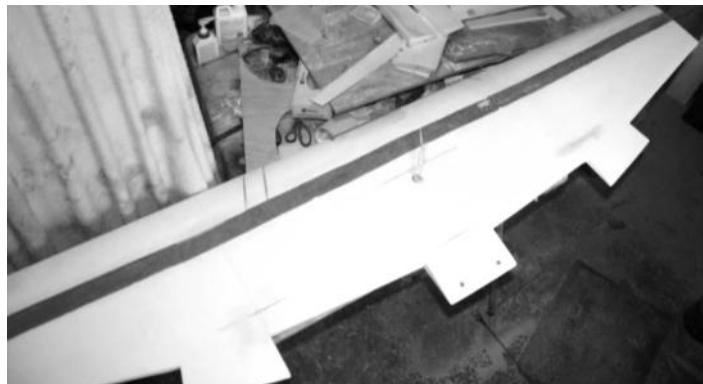
Next job was to slop some paint on and although the plan is to keep the paint to a minimum I used a high build primer to help cover the carbon spar and kept the base coats of colour and a clear top coat to just one thin coat to protect it from the glow fuel. Next step was to fit all the control surfaces, these all use Dubro nylon hinges and are fitted with steel horns and ball joints to steel clevises at the servo end.
